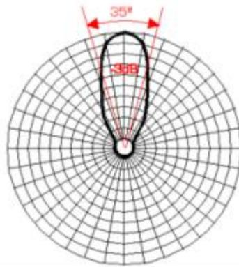
As shown above, the HPBW is the angle from where the gain, relative to maximum drops by 3dB, either side of the boresight. In the above example, the HPBW is 35 degrees. The antenna half-angle,  $\alpha$  is also defined. This is  $\alpha = \text{HPBW}/2$  i.e. 17.5 degrees in the figure above.
