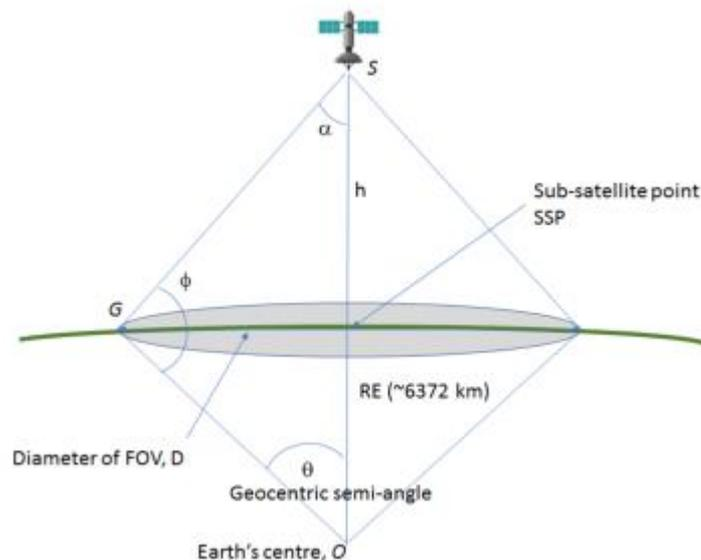
The satellite is orbiting at a height  $h$  above the Earth's surface and is therefore a total distance of  $RE+h$  from the Earth's centre,  $O$ . For the Nadir-pointing case, a triangle  $OGS$  is formed with angles of antenna half-angle  $\alpha$ , the enclosed angle  $\phi$  and the Geocentric semi-angle  $\theta$ .  $G$  is a point on the ground. We want to calculate the diameter of the Field of View (FoV),  $D$  for a given height  $h$  and antenna half-angle,  $\alpha$ . We can write,
