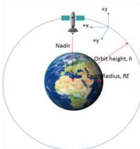
When the satellite's sensor (e.g. an antenna) is positioned with an off-Nadir angle, the antenna is slewed by an angle  $s$  relative to Nadir, in the  $x$ - $z$  plane as shown below.
