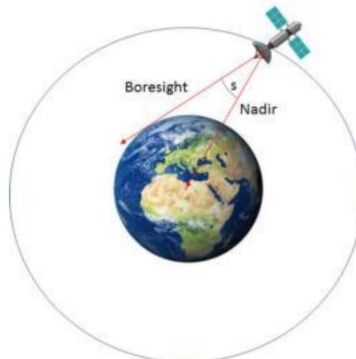
The slewing of the antenna may be achieved by means of a fixed or movable orientation of the antenna itself relative to the spacecraft or, (especially in the case of very small satellites), by moving the entire satellite so that its antenna is orientated in the desired direction.
